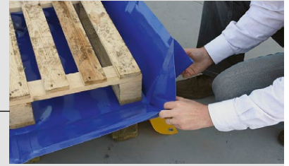
Detail of collapsing the corners
