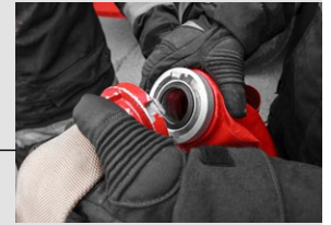
C52 Coupling (aluminium)
