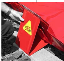
Correct anchoring of the side support
