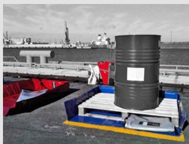
The corners are not sealed and so the tarp can easily fold around the pallet
