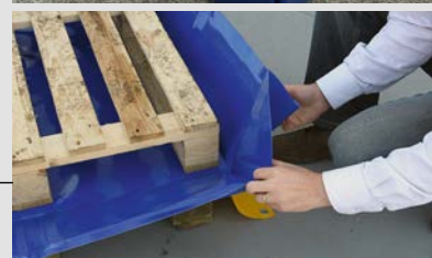
Detail of collapsing the corners
