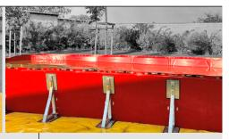
The side walls of the container can only be finally assembled after the car is placed in the container area. Then the container is filled and the car is flooded.
