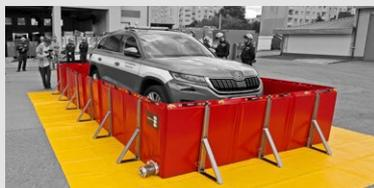
Container prepared for flooding of the car
