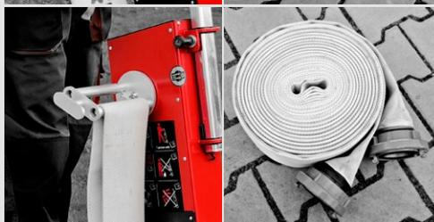
Winding the hose secured by the coupling
