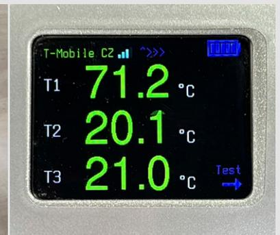
Temperature limit, overrun alarm – the device is sending a warning SMS
