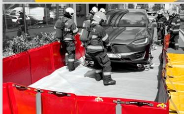
Placement of a damaged electric vehicle into the quarantine container
