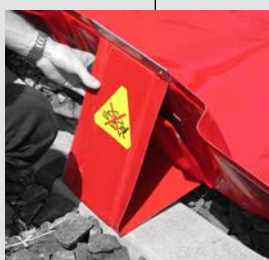
Correct anchoring of the side support
